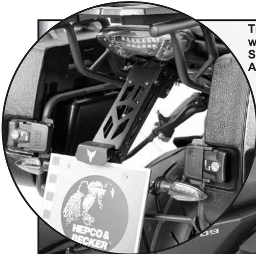
The side carrier can also be fitted in connection with the OEM licence plate holder (long version)
