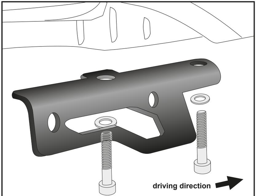
Fitting the mounting adapter front
